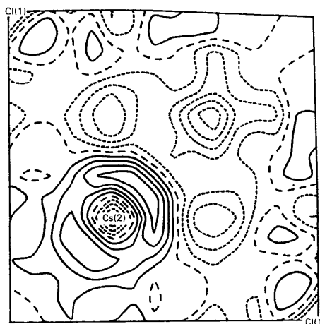
Fig. 1. Deformation charge density map for the z = 0 plane of Cs 3 CoCl 5 , containing Cl(1) and Cs(2). The contour interval in this and subsequent maps is 0.2 e \text{ \AA}^{-3} ; solid lines for positive, dashed lines for negative density. The plane extends from x = 0 to 0.5 and from y = 0 to 0.5 , downwards, the complete unique area in the plane.
